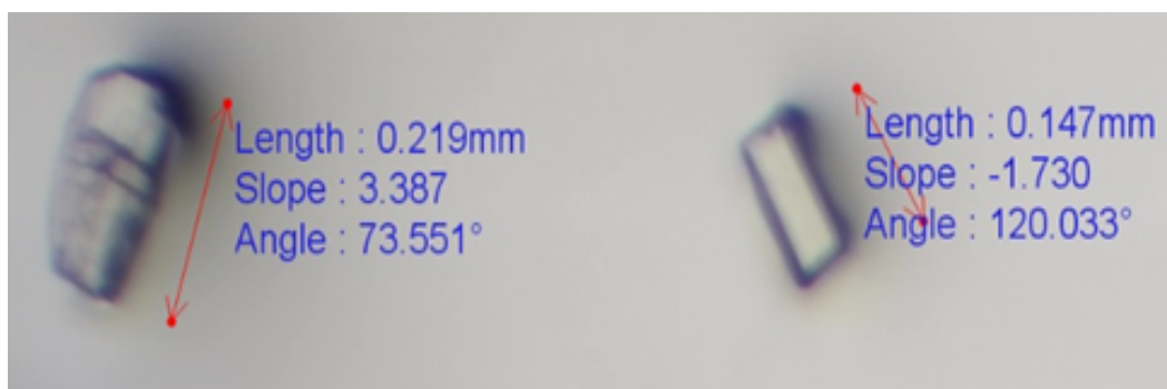
Figure 2. Left- An image of more amorphous crystals. Right- An image of a high-quality single crystal that would be ideal for SCXRD analysis. The single crystal is a similar size to the degraded crystal.
