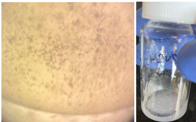
Figure 15. Left- Microscope image of polypropylene pellet placed in RV22 conditions. Right- Image of poly(acrylic acid) placed in Compound 1 conditions.
